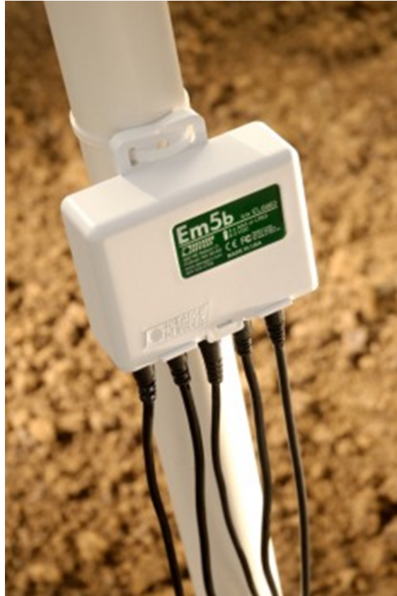
Figure 2.5 Decagon - em5b Data-logger
